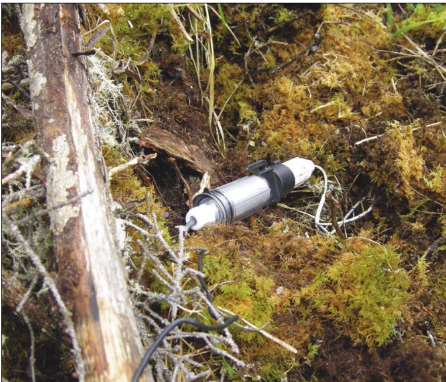
FIGURE 4 Connecting to a below-ground permafrost monitoring probe.
